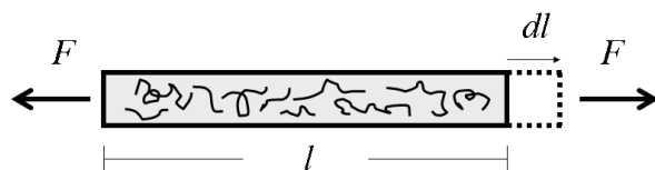
FIGURE 13. Uniaxial loading (Force F ) and extension ( l \rightarrow l + dl ) of a strip. The composition of the material is not further specified, but homogeneous.
