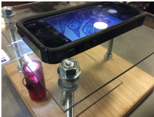
FIG. 4: $10 microscope used in General Biology laboratory course
