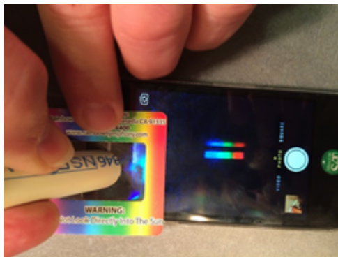
FIG. 2: General Chemistry cell phone spectroscope
