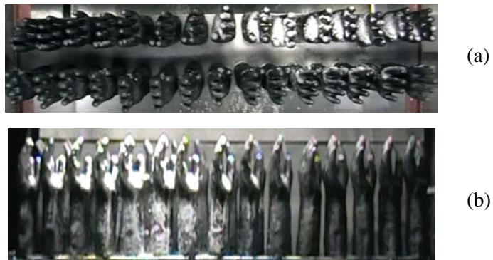
FIG. 11: Experimental flock accretion on the Pattern-L glove surface of the SM40B model: (a) top-view and (b) side-view
