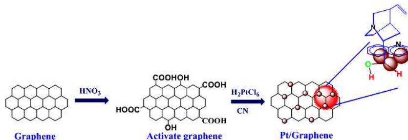
FIG. 2: Typical preparation method of Pt/graphene
