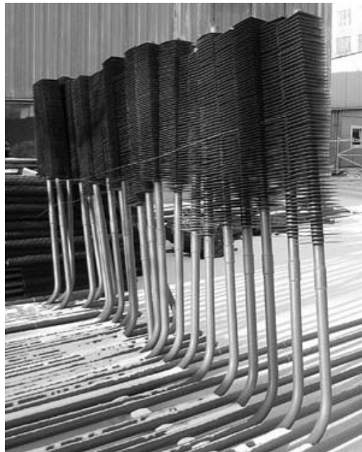
FIG. 8: Seasonal cooling devices of horizontal type
