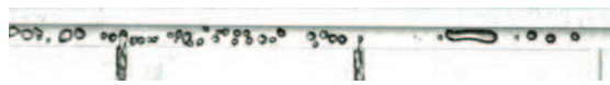
FIG. 4: An example of bubbly flow in a header at higher bubble number density.
