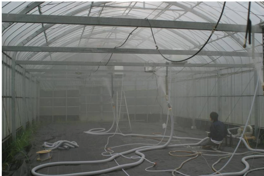
FIG. 5: The inside of the greenhouse under air-cooling testing.
