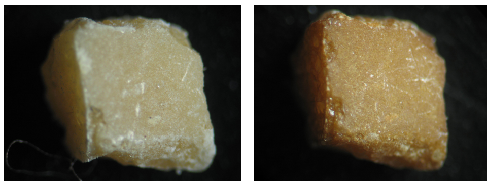
FIG. 6: Microscopic photographs of a GIM piece before (left) and after (right) a 48-h photolysis.
