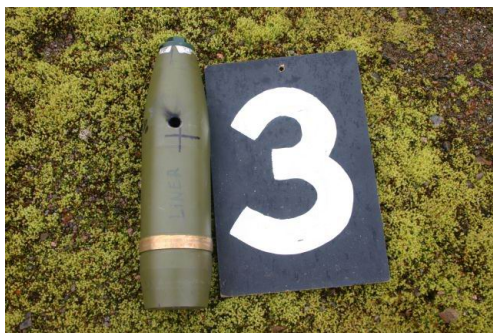
FIG. 1: Bullet impact result on GIM explosive.
