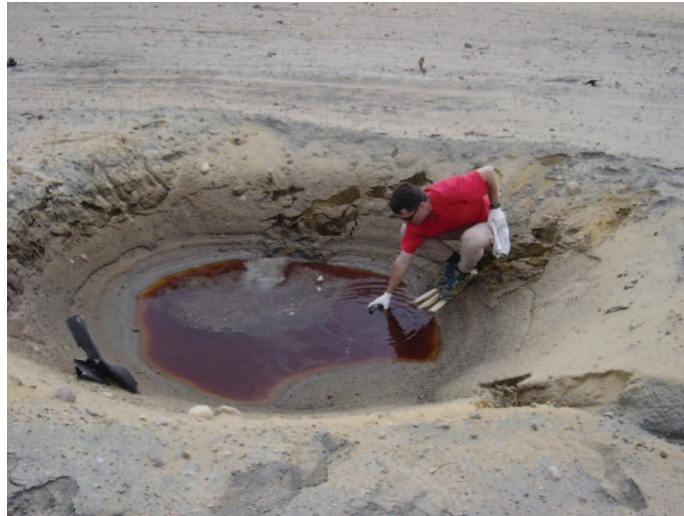
FIG. 7: Low-order detonation crater in Cold Lake RTA.
