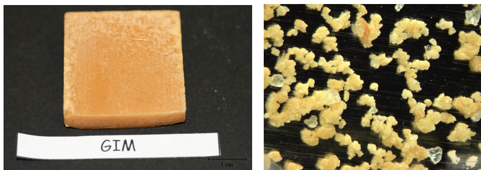
FIG. 7: GIM explosive before (left) and after grinding (right).
