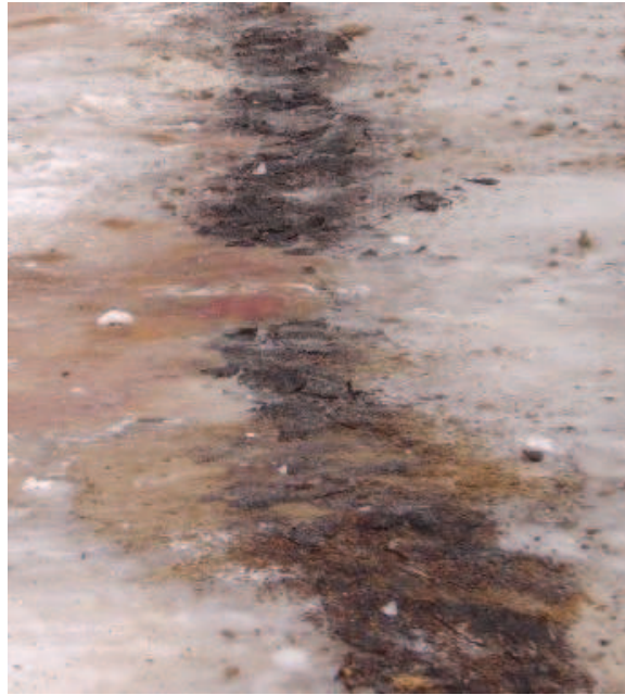
FIG. 6: Leftover residues after burning on snow.
