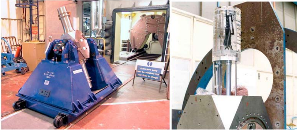
Fig. 2. The Rotating Heat Transfer Rig used by Rolls-Royce to study the effect of rotation on blade.
